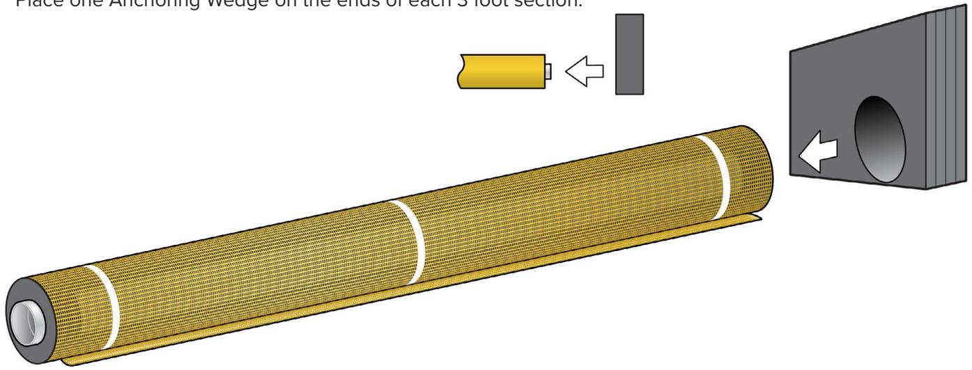
2. Connect together two sections of the CurbGuard Plus by inserting the Male Pipe Connector into the open end of the Female Pipe Fitting. (gluing the sections together using PVC cement is optional)
