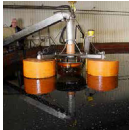
Equipment: Ultra-SurfCleaner Capacity: 8,000 liters (2,113 gal) per hour Purchased: 2004
